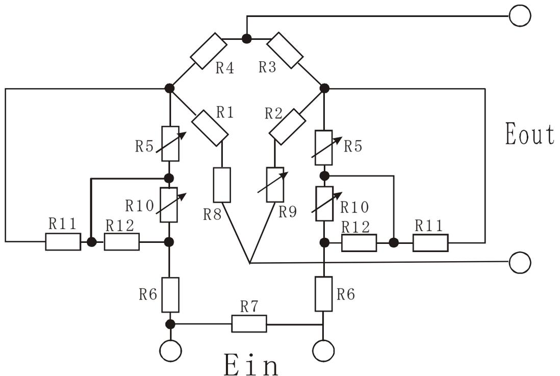
**Figure 2.13.** Load cell circuit
