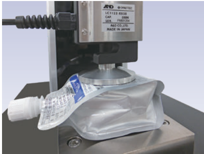
Packing container compressive strength test
