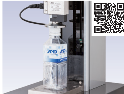
Plastic bottle compressive strength test
